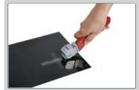
step 1: make grid cutting on surface
